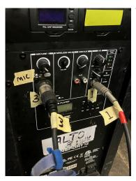
This is the master speaker, where you connect the microphone and control the volume.
